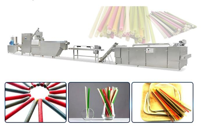
2. Production process: raw material configuration--raw material mixing--extrusion molding--hot air drying--cutting
