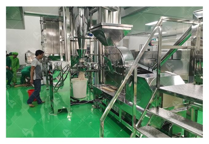
Drying is crucial for stabilizing the quality of the final product. Modern drying equipment uses multizone control, automatically adjusting the drying curve based on changes in product moisture content. A specially designed belt system ensures more uniform heating of the product, avoiding
