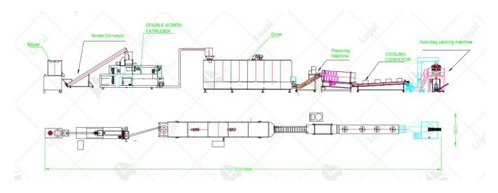
Our machines can place flexibly according to the size and the dimension of factory. Our machines can be placed not only straight but also bent.
