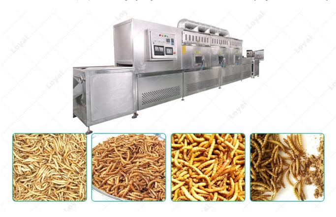
Microwave mealworm drying equipment is used for drying mealworm by microwave, which has many outstanding advantages over conventional methods: such as greatly shortened processing time, easy control, good product quality, straight insects, high degree of expansion, maintain color and freshness, low loss of water and nutrients, low bacteria content, high treatment efficiency, low cost, low energy consumption, small floor space, improved working conditions and environmental sanitation.
