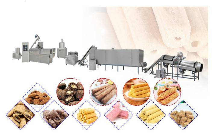
The core filling snack making equipment produced by Shandong Loyal is composed of powder mixer, screw conveyor, twin screw extruder, sandwich machine, shaping machine, elevator, electric oven, and automatic seasoning machine. Among them, the powder mixer is generally used to mix and prepare various powders. And it can also be used for the preparation of raw materials. Shorten the manual mixing time, save time and effort.
