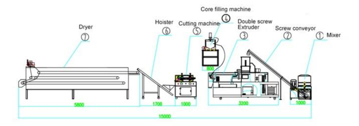
Using the unequal-distance non-standard screw system of the extrusion, the gas in the material is discharged and quickly filled with the material. The material is subjected to the shearing force to produce backflow, which increases the pressure in the chamber. The friction between the stack and the chamber makes the materials fully mixed, squeezed, heated, glued, and gelatinized to produce organizational changes, and the original structure is destroyed.
