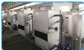
Closed cooling tower
