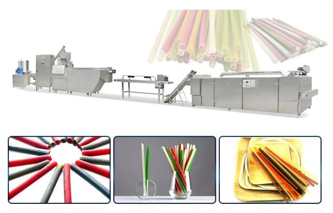
The edible straw production line mainly uses rice, cassava rice noodles, etc. As raw materials using an extrusion molding process to produce secondary puffed foods of various shapes on the market. Rice straw production line has reasonable design, high degree of automation, precise control of extrusion parameters, and the main engine is equipped with high and low pressure screws, which increases the use range of raw materials, reduces costs, and improves product quality.
